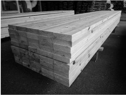
[梁材（構造用製材）100m<sup>3</sup>]
